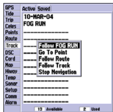
The track name automatically appears when highlighted on the 'Saved' list and NAV is pressed.
